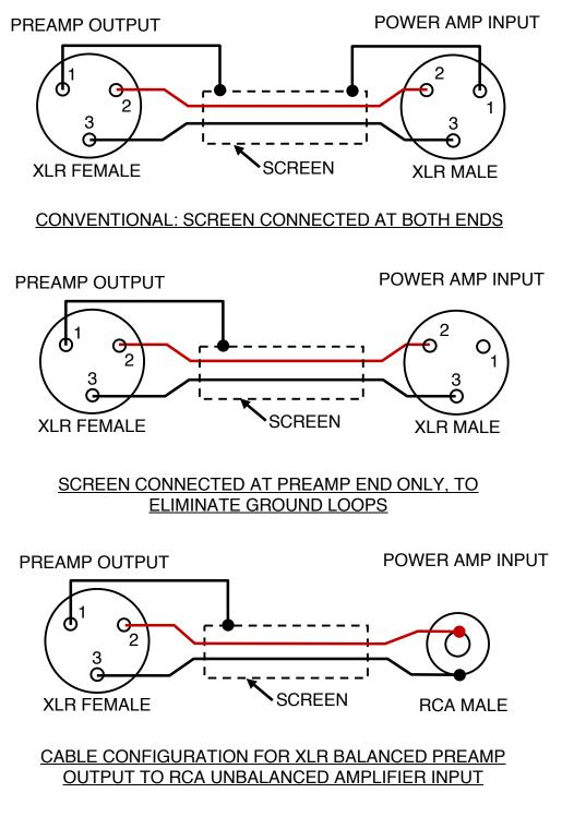
When connecting the XLR / BALANCED outputs to an amplifier with an RCA / Single Ended input, the switch must be set to the 'SINGLE ENDED' position. Once all the connections are completed and checked, ensure that the volume control is at the minimum setting (rotated all the way left).
